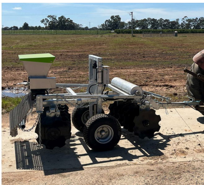
Left: GreenPro 6in1 Seeder used for this project purchased by FGV. Right: Direct Drill kit attached
