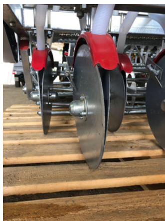
Left: Network Seeder Double Disc opening assembly. Middle: Network Seeder (10 row) Right: Taege Vineyard Drill
